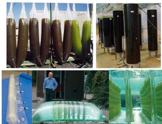
Polyethylene bags and Annular Columns. Top left: Polyethylene bags at Necton, SA – Algarve, Portugal; Top right: Annular Columns at Department of Agricultural Biotechnology of the University of Florence, Italy; Bottom: Inflatable bags with multiple vertical panes (Proviron, Belgium).
