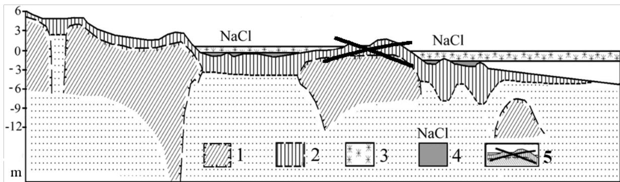
**Figure 1:** Geocryological cross-section of Yamal coast of Baydaratskaya Bay, Kara Sea: 1 – permafrost; 2 – seasonally frozen (thawed) sediments; 3 – sea ice, 4 – cryopeg, 5 – seasonally thawed layer removal.
